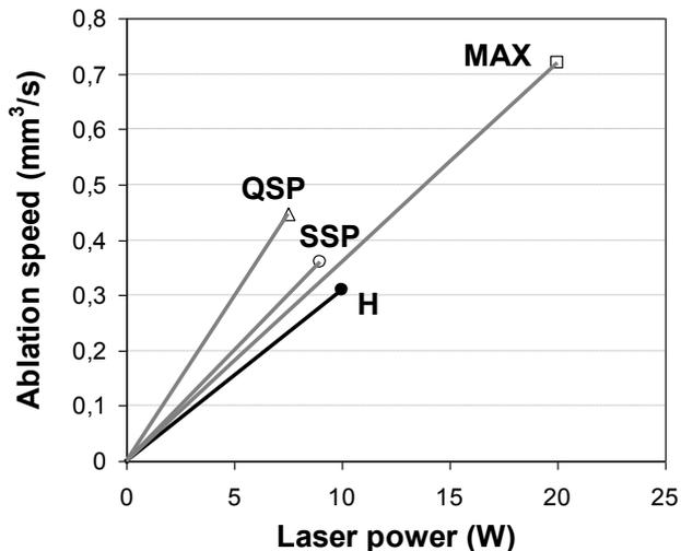
Fig. 5: Ablation speed in enamel for the QSP, SSP and MAX modes of the Er:YAG laser (Fidelis/LightWalker), and for the H mode of the Er,Cr:YSGG laser (WaterLase iPlus). The lines extend to the maximum available laser power for a particular laser mode. The data for the QSP and MAX modes is taken from refs. [25] and [17], respectively.
