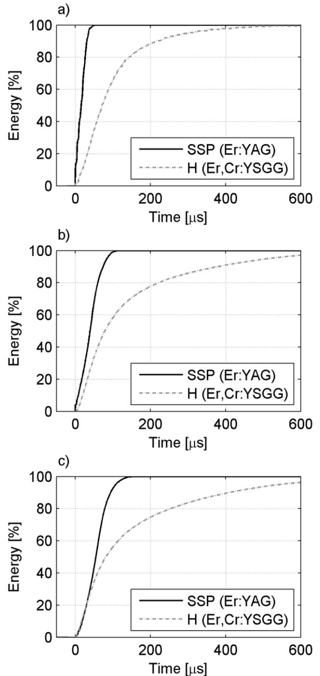
Fig. 3: Temporal development of the cumulative output laser energy for Er:YAG (SSP mode; Fidelis/LightWalker) and Er,Cr:YSGG (H mode; WaterLase iPlus). Temporal developments are shown for different total delivered (100%) output laser energies of a) 20 mJ; b) 100 mJ; and c) 300 mJ.
