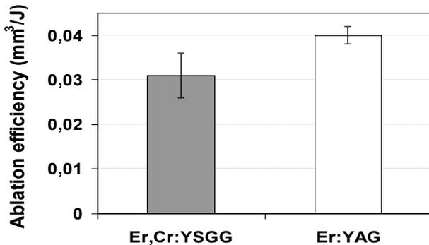
Fig. 4: Measured ablation efficiency in enamel for the Er:YAG (SSP mode; Fidelis/LightWalker) and Er,Cr:YSGG (H mode; WaterLase iPlus) laser wavelengths.
