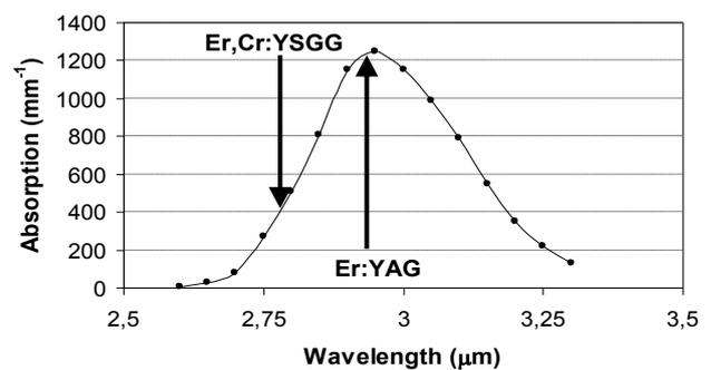
Fig. 1: The absorption curve of water in the middle infrared region. The plot shows the position of the two dental laser wavelengths used for hard-tissue ablation: Er,Cr:YSGG (2.79 micrometers), and Er:YAG (2.94 micrometers). The figure is reprinted with permission from reference [7].
