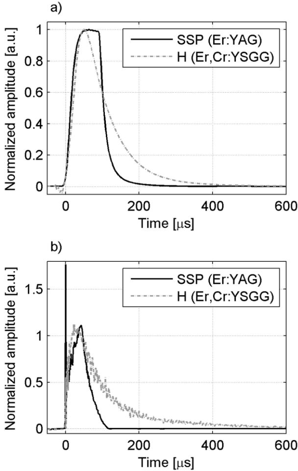
Fig. 2: Measured a) flash-lamp pump pulse and b) laser output pulse shapes for Er:YAG (Fidelis/LightWalker) and Er,Cr:YSGG (WaterLase iPlus) at the output energy of 100 mJ. The pulse shapes represent an average of 46 pulses.
