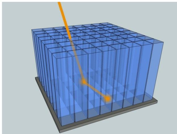
Fig. 1: Inelastic scattering of a gamma photon, followed by photoelectric absorption, serves as a precise relative temporal marker for any pair of 64 readout channels in a TOF PET detection block.
